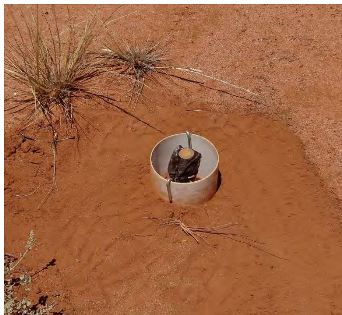
A collar fitted to a CPE to orientate the foxes head over the bait to reduce bait removal without the ejector being activated.
